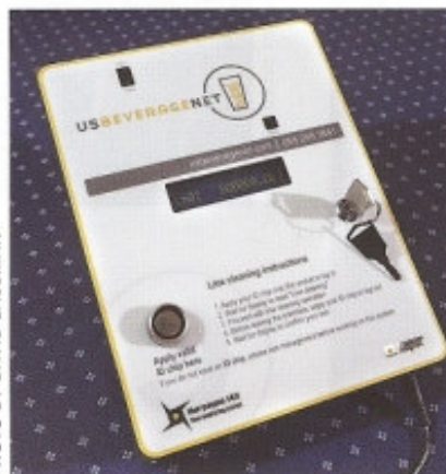
The US Beverage Net flow-monitoring system measures how much beer is poured from the taps against how much money goes into the cash register.
