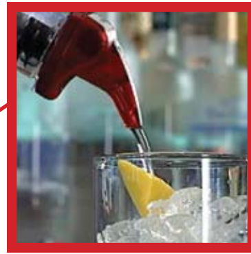
● Radio frequency identification (RFID) tags on Capton Inc. pour spouts measure bottle tilt, pour duration and flow rate; the data is transmitted wirelessly and analyzed against information about the brand's viscosity and bottle shape and size to determine the amount poured.
